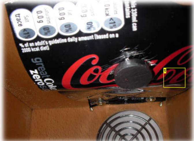
Image Notes 1. The magnet glued to the coke can with epoxy.
